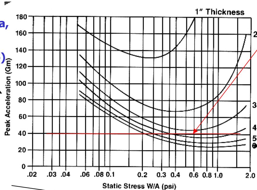
Polyethylene, 2 pcf, 36" Drop Height Shock Cushion Curves
